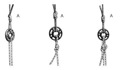
**Figure 1.** Moving: A single rope passed through the anchor in a moving rope setup.
