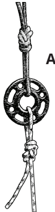
Figure 2. Single stationary: A single rope attached using a retraced figure-8 knot in a stationary rope setup.
